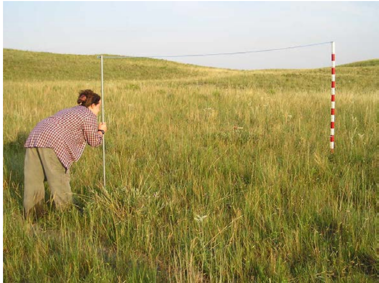
The proper use of a Robel Pole to measure Visual Obstruction Reading (VOR), a measure of grass density and biomass. Photo by Silka Kempema.
